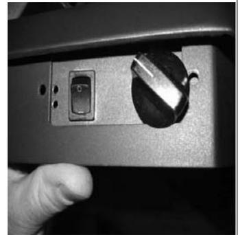
6) Route cable from speed control to fan and reattach wire support tabs on the underside of the ash lip. Note wire positions. (Fig.18 & Fig.19)
