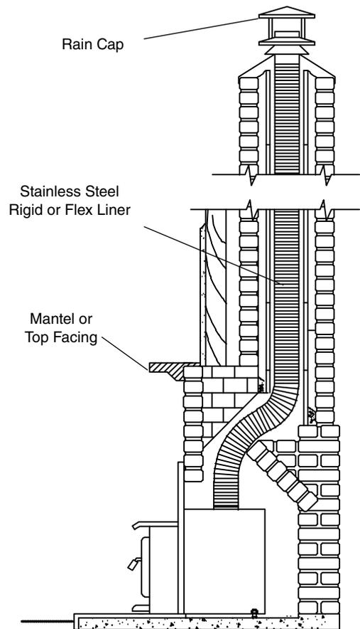
**Pacific Energy highly recommends the use of a full liner as the safest installation and providing optimum performance. When connected to a full liner, the Insert is able to draft correctly and will prevent problems such as difficult start-ups and smoking out the door.**
